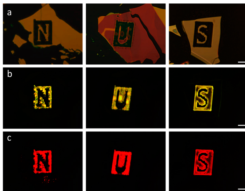
Figure 5. Colorful micropatterns on phosphorene. (a) Optical images of the fabricated micropattern “NUS”. (b and c) FM images of the created micropatterns showing different fluorescence colors when excited by blue (460–490 nm) and green light (510–550 nm), respectively. Scale bar = 10 \mu\text{m} .
